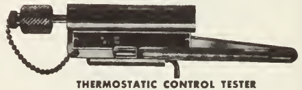
6-22. A thermostatic testing unit. The refrigerant cylinder connects to the knurled nut on the left. The control thermal bulb fastens to the tester just back of the mercury bulb of the horizontal thermometer.
